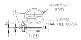
NOTES: 1- FOR CHEMICAL APPLICATIONS USE STAINLESS STEEL EQUIVALENTS FOR FASTENERS AND EXPANDED PTFE FOR GASKET.
